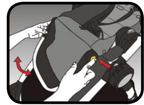
**2** To raise or lower footwell: Press buttons on upper portion of footwell and pull up or push down until it clicks into the desired position.
