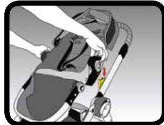
**2** Locate desired seat position on stroller frame. Align seat adaptor brackets with mounting brackets on stroller frame.
